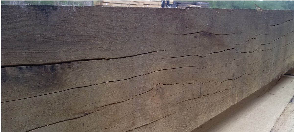
Drying fissures in air dried beam
