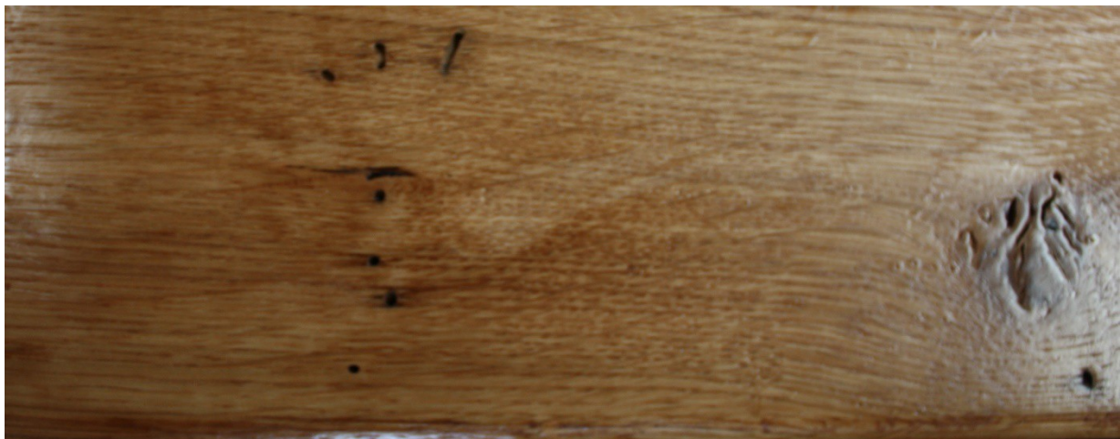
Black ambrosia tunnels in an oak decking board.
